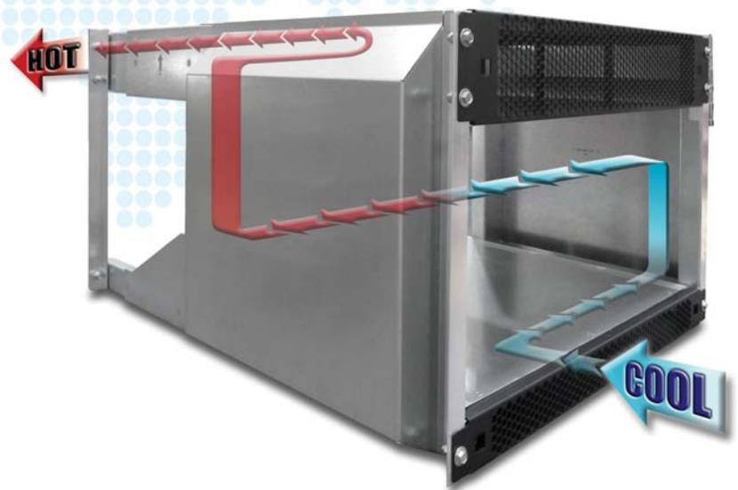
Figure 1: Using a series of air baffles, cool air is drawn in from the front of the rack and redirected to the equipment intake on the side of the unit, then exhausted to the rear of a rack.
