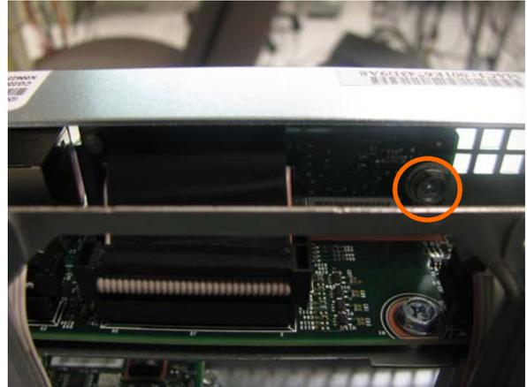
22. Removal of the Front Control Panel does not require any tools.
