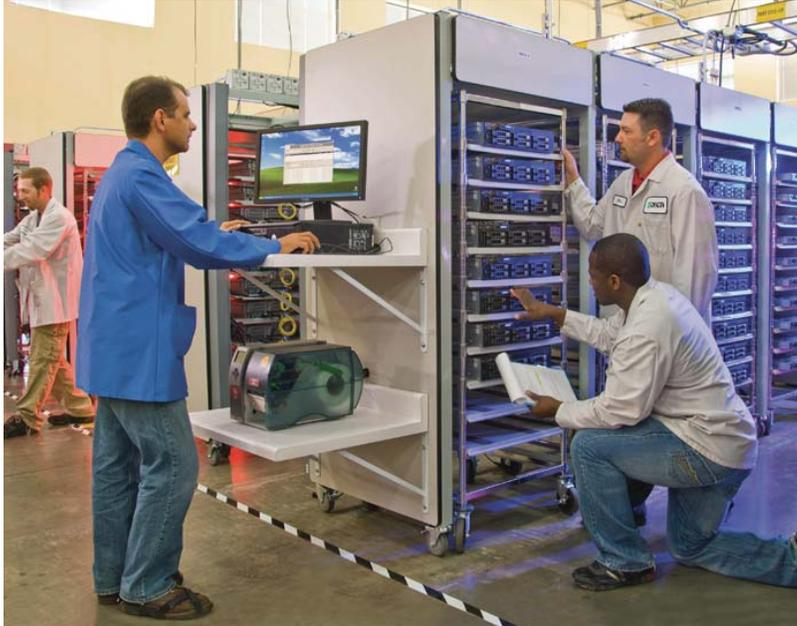
**FIGURE 5:** Engineers testing individual systems prior to rack integration to ensure each system complies with requirements.
