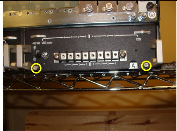
Removal of the top metal cover on PEM A and PEM B requires a T9 Torx Screwdriver.
